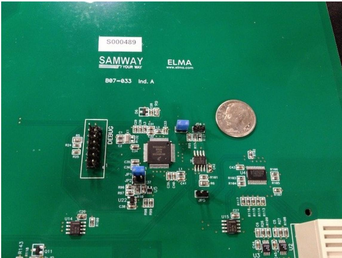
**Figure 1** shows the Elma IPMI controller surrounded by other components. Less than the size of a dime, the controller delivers IPMI functionality for newly developed modules.
